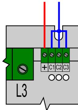
Figure 6: Linking of C1, C2 and C3
