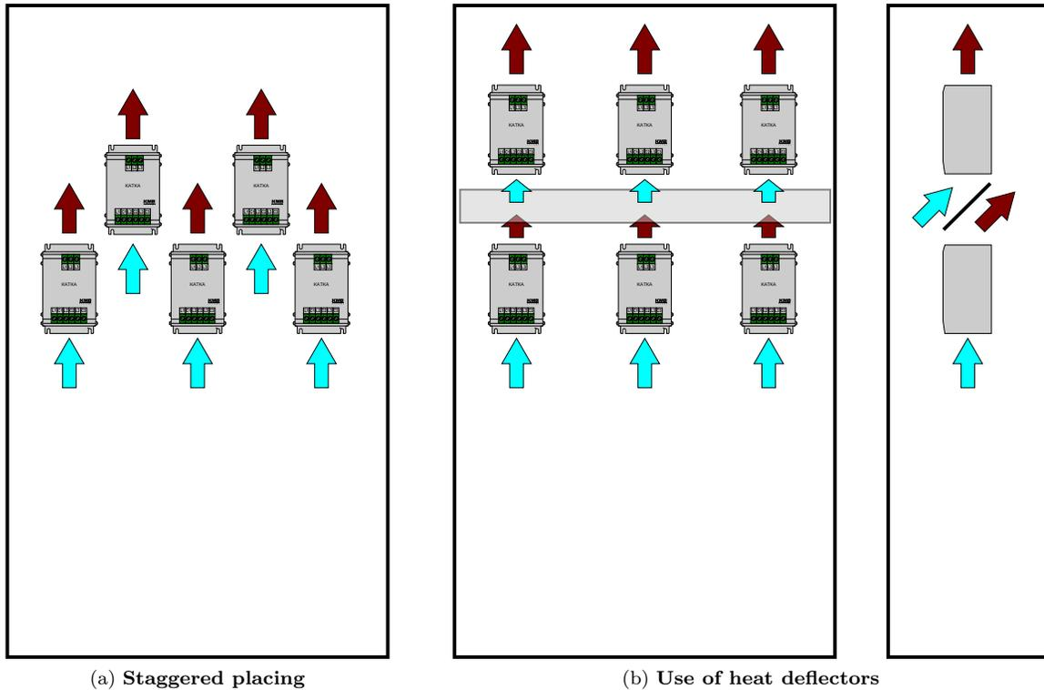
Figure 3: Installation example
