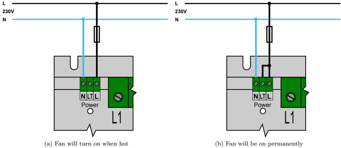
Figure 1: Connection of fan supply voltage to KATKA 80
