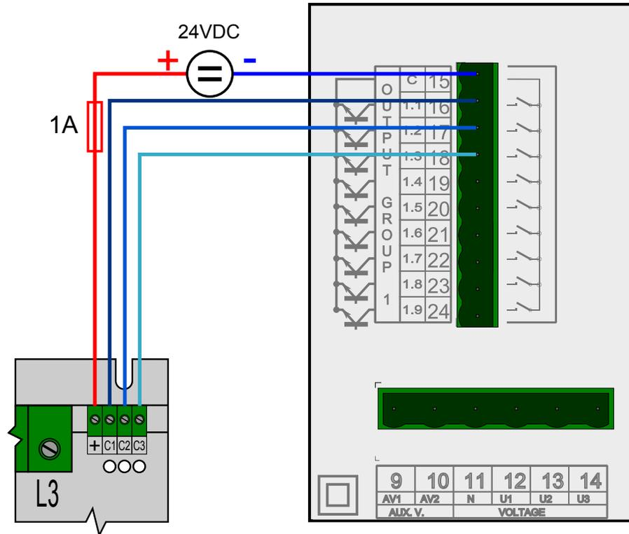
Figure 5: Connection of control signal
