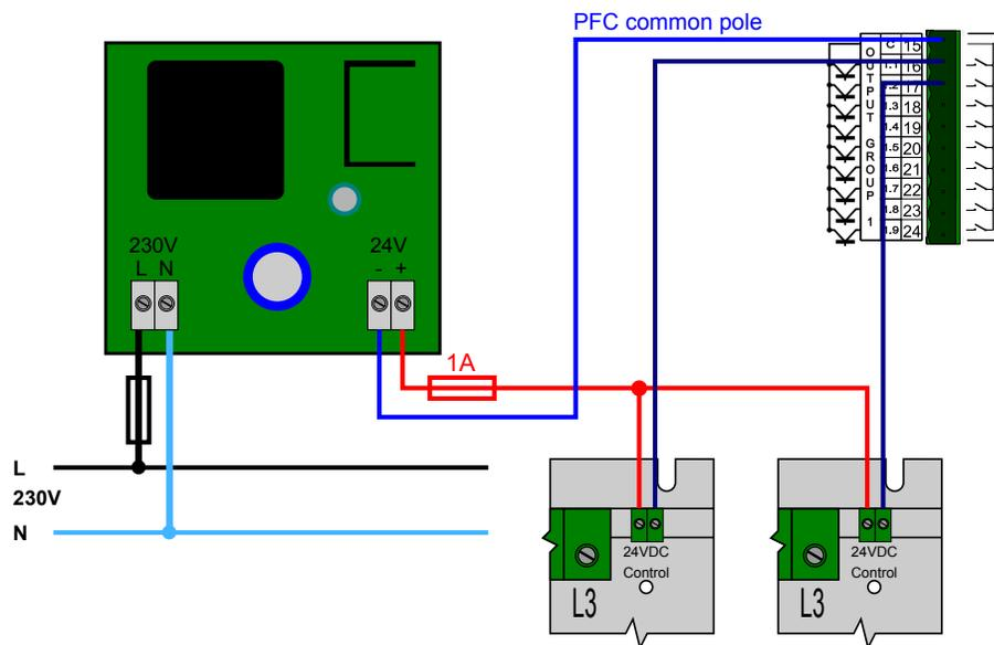
Figure 8: Possible connection of ZP24
